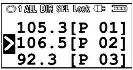
The preset FM frequencies and preset numbers are shown. Preset numbers are enclosed in brackets. When moving up and down through the preset list, each successive item is preceded by a cursor .
